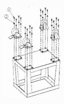
Step 2. Four handles provided will screw into the base of the oven firebox to assist in the assembly of the cart.
