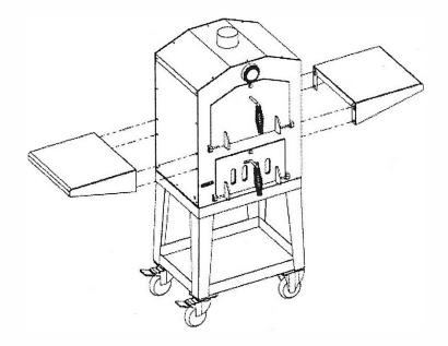
Step 4. Insert the chimney and cover on the top of pizza oven. No screws are needed.
