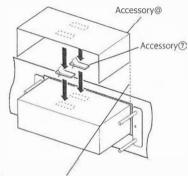
Affix the top cover tightly with no clearance between it and the mounting surface.
