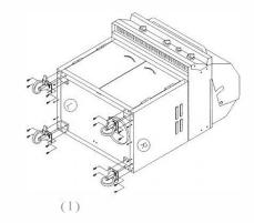
2. Assemble two side shelves by using 8 MS Hex-Philip bolts. (Four for each side shelf).
