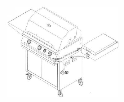
After insert thru hole of right side panel, connect to inlet of grill head located on the right bottom of control panel.
