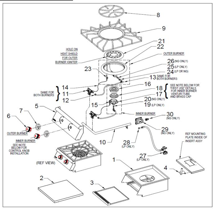
NOTE: After opening the main box, you will find 3 smaller boxes that contain the following items to be installed per drawing at right: Venturi Tube Cap and Brass Tube (Inner Burner) and Control Panel Knobs
