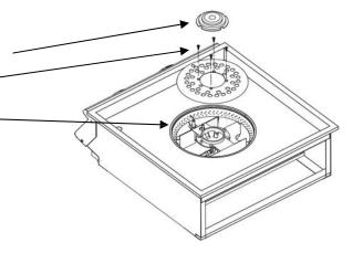
STEP 3 / Per the drawing below. Carefully unplug the red electrical leads by pinching the lead's metal connector with your fingers and gently pull straight down until it releases from the igniter (Avoid twisting the lead to prevent damaging the ignitor) from both igniters and tuck them out of the way. Note, the lead for the Center Burner shown routed through the bracket opening when you move it. Note, there's no need to remove the igniters.
