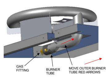
3. Rotate the Outer Burner towards the slot provided until you can slide the Outer Burner out of the Power
