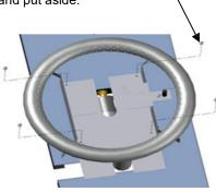
2. Slide the Outer Burner Tube until it clears the gas
