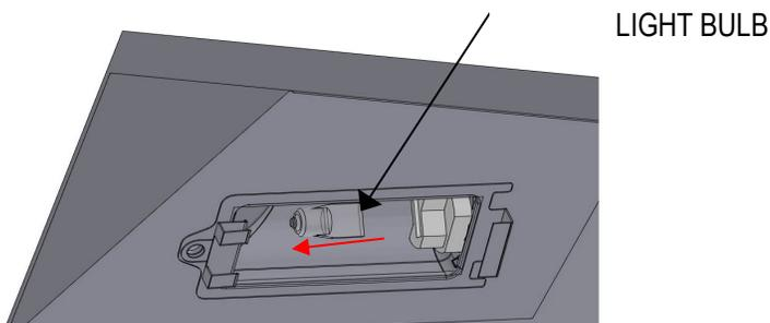
4) Using a soft cloth or paper towel, replace new light bulb into the housing (fingerprints left on the bulb may reduce its life). Make sure the metal prongs on the light bulb slip into the openings in the light housing
