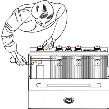
The provided Lighting Rod is for holding a fireplace match to light the grill. Is located inside the front of the grease tray as shown below.
