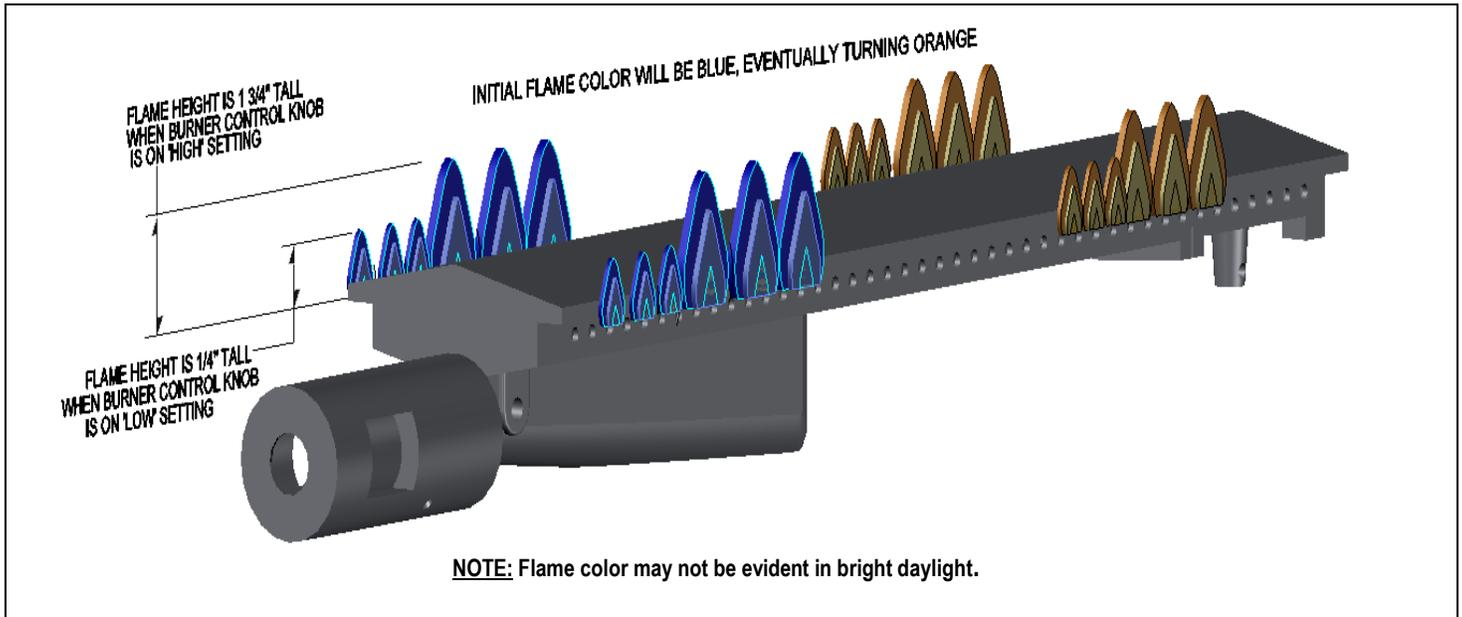
9) **NOTE:** If igniters fail to produce a spark at the electrode tip, burners can be manually lit with a fireplace-type match. See next page for instructions.
