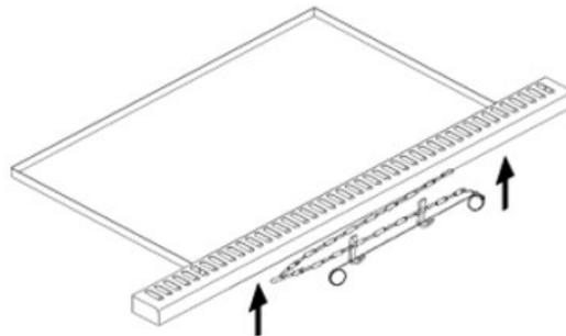
**INFRARED "BACK BURNER"** The rear Infrared Back Burner allows for slow rotisserie cooking of meats and poultry. Infrared burners radiate heat onto the outer surface of the food. This allows cooking without the grease drippings burning on the flame tamers
