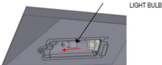
4) Using a soft cloth or paper towel, replace new light bulb into the housing (fingerprints left on the bulb may reduce its life). Make sure the metal prongs on the light bulb slip into the openings in the light housing
