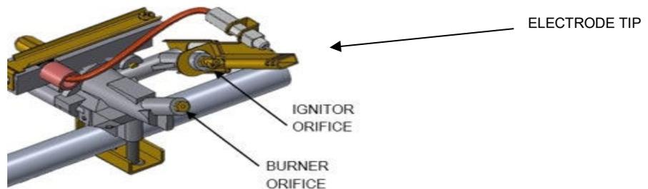
**MISALIGNMENT OF IGNITER ON BURNER / CORRECTION**
