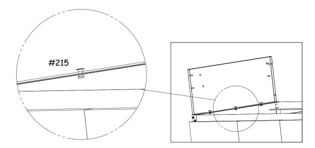
3 Place Diablo Grill Head on cart bottom and secure to side adapters using screws indicated
