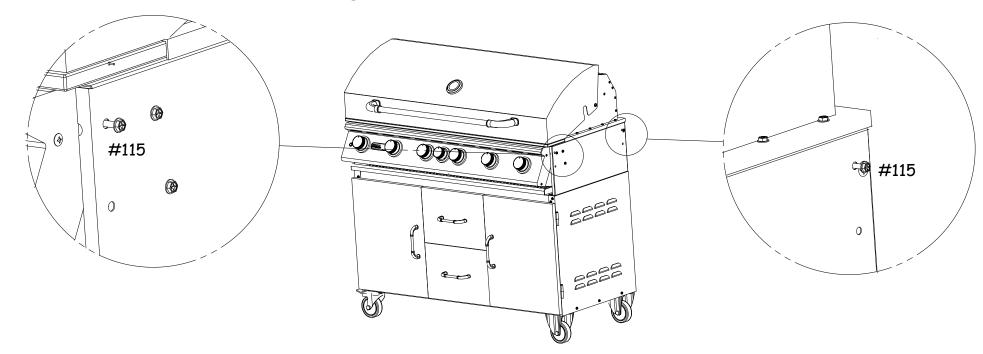
6 Slide the side shelf over the screws and tighten. Add #115 and #130 as shown to secure shelf.
