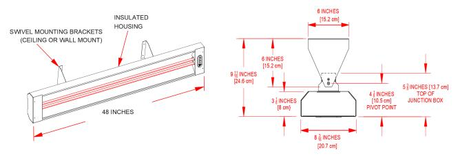
Heater must be installed with the quartz tube horizontally level. For maximum tube life, use a carpenter's level tool to find the optimum level position for the heater's body. It's important to always maintain the minimum clearances from the heater body to any combustible materials.
