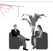
Install fixture to heat the area from the "cold side" if possible. This helps compensate for increased body heat losses due to exposure. Warm floors reradiate heat. Warmer air rises from floor. Some heat reflects from floor. Mounting a heater directly over a table or other obstruction will block the energy, primarily heating the object. It is best to move heater to the side, allowing complete body and floor coverage. OUTDOORS
