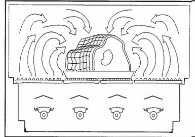
**Flare-Ups:** The fats and juices that drip from the meat cause flare-ups. Since flare-ups impart the distinctive taste and color for food cooked over an open flame, they should be expected and encouraged within reason. Nevertheless, uncontrolled flaring can result in a ruined meal. To control excessive flare-ups caused by too high a heat setting, turn the heat control knob to a lower setting.
